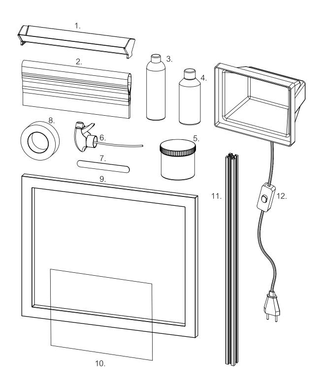
1.Scoop coater 2.Printing squeegee 3.Emulsion 4.Emulsion remover 5.Ink 6.Trigger Sprayer lid 7.Stiring stick(\*3) 8.Masking 9.Screen 50x40
