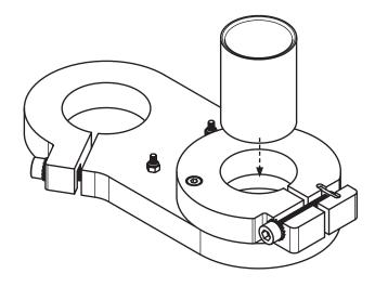
Assemble the magnets on the last Plexiglas part as shown with the two M3x10 screws.
